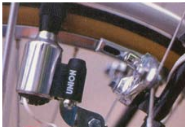
A dynamo converts mechanical energy into electrical energy.
