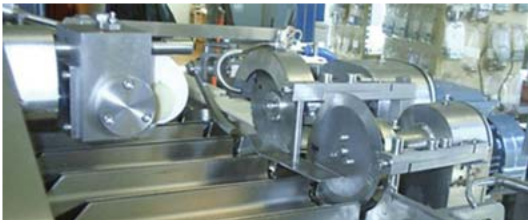
Grinding is a commonly used method for removing the excess material from the castings, forgings and weldments
