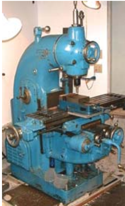
Milling machine is used for dressing surfaces by rotary cutters.
