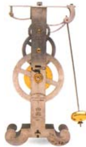
A pendulum clock designed by Galileo. Galileo was the first to design a clock based on the relationship between gravitational force ( g ), length of the pendulum ( l ) and time of oscillation ( t ).
