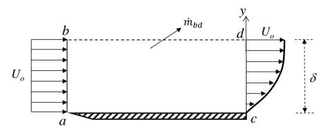
The ratio of the mass flow rate,  $\dot{m}_{bd}$ , leaving through the horizontal section *b*-*d* to that entering through the vertical section *a*-*b* is \_\_\_\_\_
