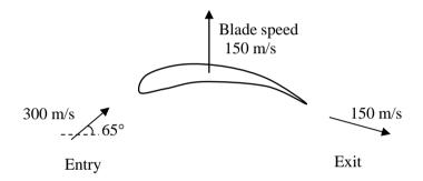
The magnitude of absolute velocity at entry is 300 m/s at an angle of  $65^{\circ}$  to the axial direction, while the magnitude of the absolute velocity at exit is 150 m/s. The exit velocity vector has a component in the downward direction. Given that the axial (horizontal) velocity is the same at entry and exit, the specific work (in kJ/kg) is\_\_\_\_\_
