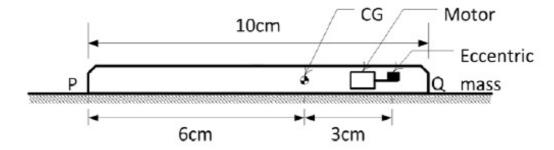
Given in addition that the eccentric mass = 2 grams, eccentricity = 2.19 mm, mass of the mobile = 90 grams,  $g = 9.81 \text{ m/s}^2$ . Uniform speed of the motor in RPM for which the mobile will get just lifted off the ground at the end Q is approximately
