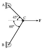
Q.48 If  $\mathbf{F} = 1 \ kN$ , the magnitude of the vertical reaction force developed at the point B in kN is
