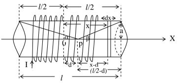
Let us consider a finite circular solenoid of radius 'a' and length 'l'. let 'n' be the no. of turns per unit length and 'I' be the carrying current. Assume that the solenoid axis coincides with the xaxis and the origin coincides with centre. Let 'p' be the point of observation at a distance 'd' from the centre.
