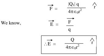
NOTE: Thus electric field intensity is independent of the amount of test charge. In Cartesian system:
