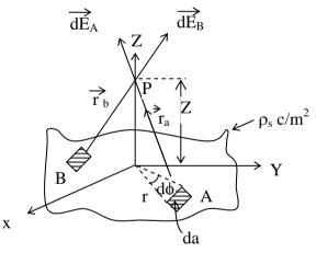
Consider two diametrically opposite elementary surface charges located at A & B. Let point of observation 'P' be along Z axis.
