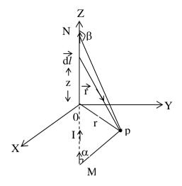
Let us consider a finite conductor of length MN, for the sake of generality  $OM \neq ON$ . Let 'p' be the point of observation on XY plane.
