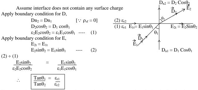
If  $\varepsilon_{r1}$ ,  $\varepsilon_{r2}$  and angle of incidence are given, angle of emergence can be calculated using the above equation.
