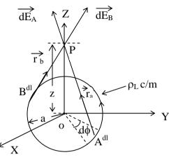
Consider two diametrically opposite elementary displacements located at A & B. Let point of observation 'P' be along 'Z' axis.
