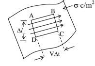
Flow of electric charges over a surface represents surface currents. Every surface current is associated with a mobile surface charge density  $\sigma c/m^2$ .
