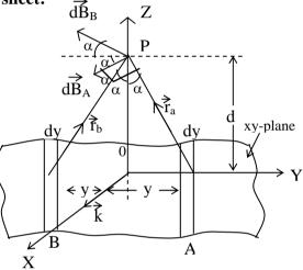
Let us consider an infinite current sheet lying on x-y plane carrying a surface current along the positive x-direction ( $\vec{K}$ ) with a surface current density K.
