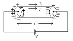
Current flowing through a conductor is directly proportional to the potential difference across it, provided temperature is kept constant.
