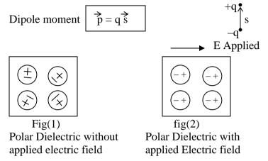
**Polar Dielectrics:** The charges in the molecules of polar type have permanent displacement from each other. The molecules have permanent dipole moment. They are randomly oriented as shown in fig(1). Net dipole moment zero until an electric field is applied.
