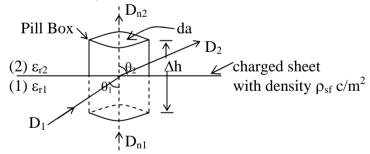
Consider a boundary formed by two dielectrics as shown in the figure. An infinite charged sheet with charge density  $\rho_s c/m^2$  is placed at the boundary. The dielectric constants of the media 1 and 2 are  $\in r_1$  and  $\in r_2$  respectively.  $\theta_1$  is the angle of incidence.  $\theta_2$  is the angle of emergence.  $D_{n1}$  and  $D_{n2}$  are the normal components of flux density vectors.
