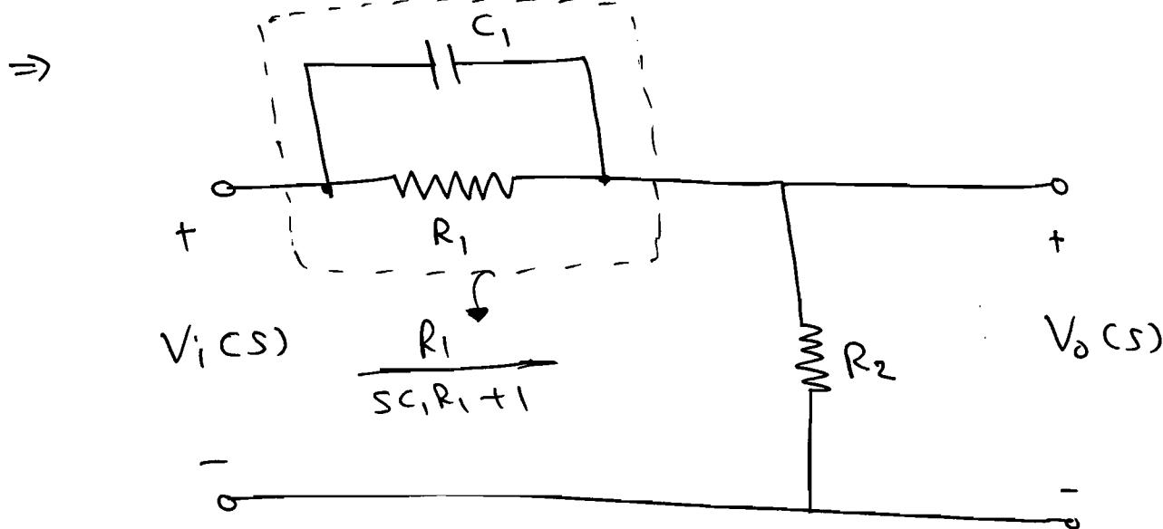
$$\Rightarrow \frac{V_o(s)}{V_i(s)} = \frac{R_2}{\frac{R_1}{sC_1R_1 + 1} + R_2}$$
