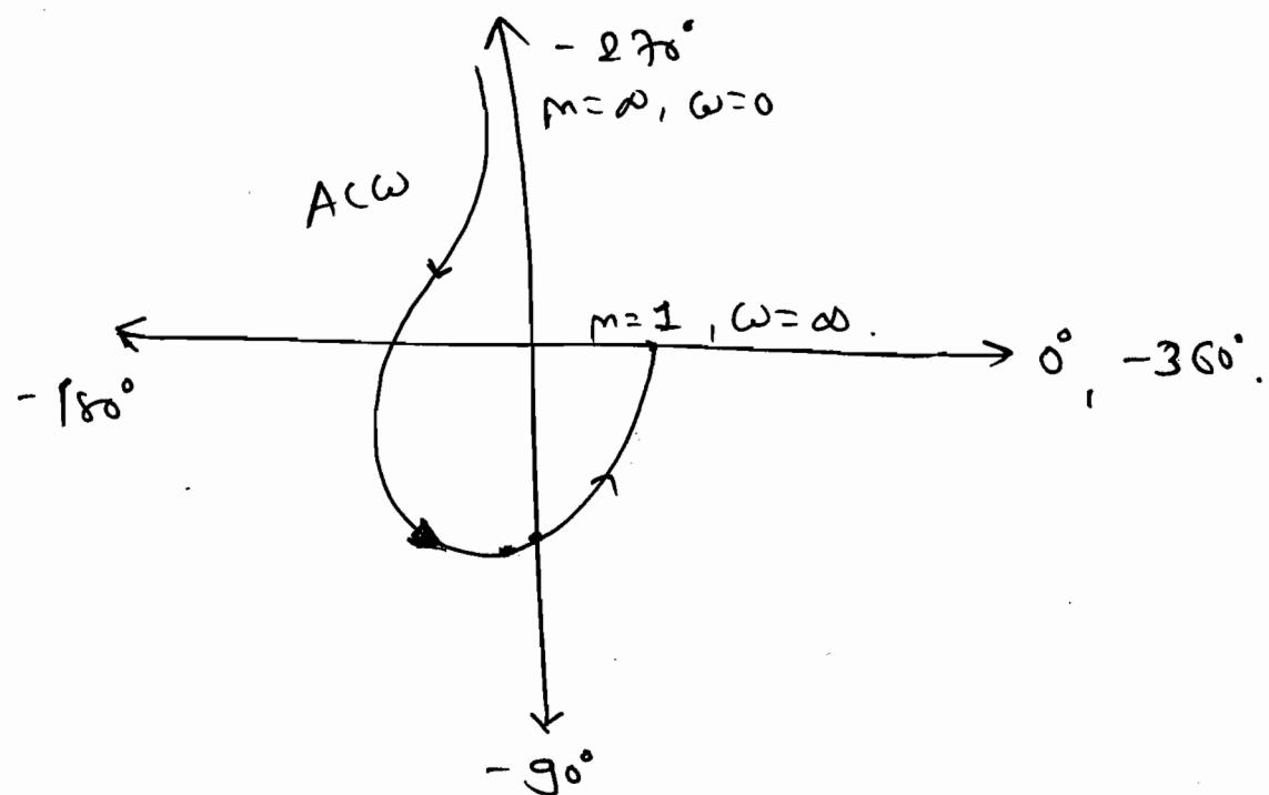
Note: The addition of each ~~line~~ finite zero shift the ending angle  $+90^\circ$  in the Anticlockwise direction.
