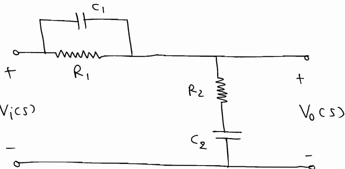
$$\text{T.F. } \frac{V_o(s)}{V_i(s)} = \left( \frac{1 + \gamma_1 s}{1 + \alpha \gamma_1 s} \right) \times \left( \frac{1 + \gamma_2 s}{1 + \beta \gamma_2 s} \right).$$
