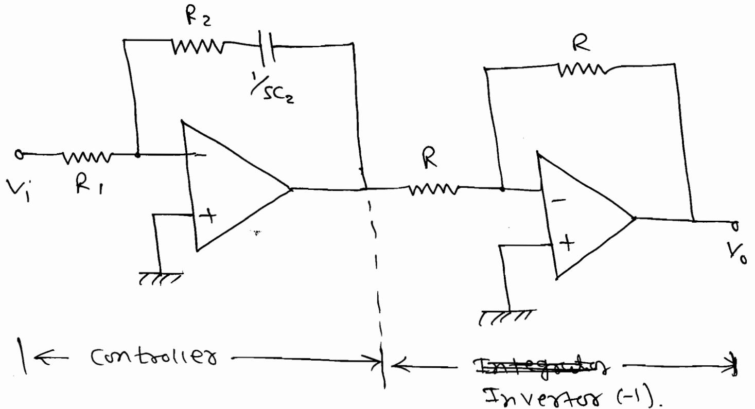
$$\therefore \frac{V_0(s)}{V_i(s)} = \frac{R_2 + \frac{1}{sC_2}}{R_1 + R + \cancel{R_2 + \frac{1}{sC_2}}}.$$
