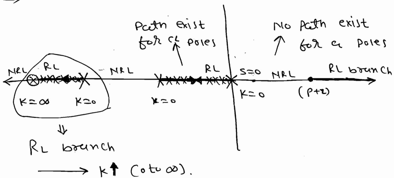
⇒ A point exist on Real axis just locus branches, the sum of the the poles and zeros to the Right hand side of that point should be odd.
