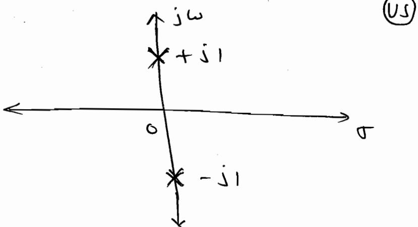
$\Rightarrow$  Whenever many times Row of Zeros occurs and all the Co-efficients in the 1<sup>st</sup> Column are positive then the system is unstable the poles must lies on the imaginary axis which are repeated.
