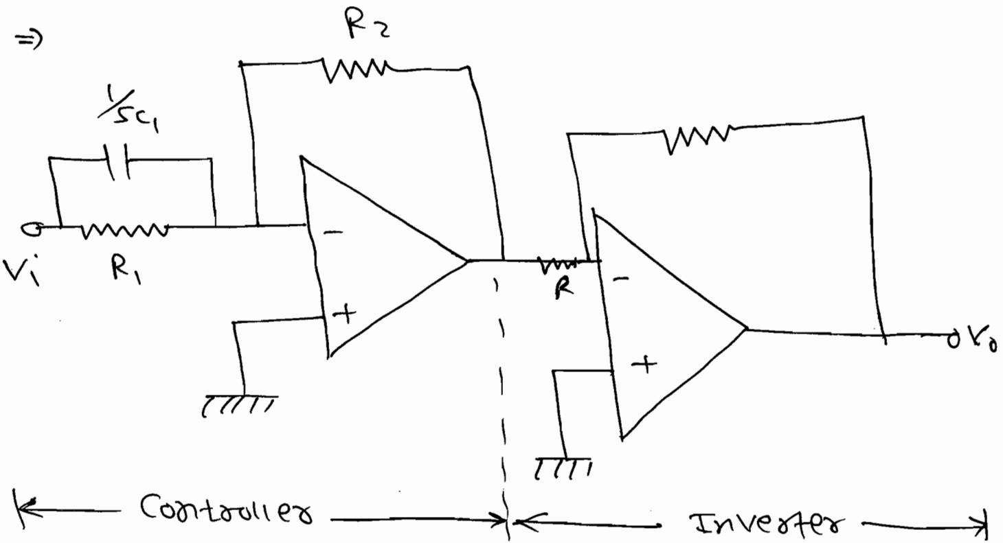
$$\Rightarrow T.F. = \frac{V_0(s)}{V_i(s)} = \frac{R_2}{R_1 + 1/\text{SC}_1} = \frac{R_2}{\frac{R_1}{1 + \text{SC}_1 R_1}}.$$
