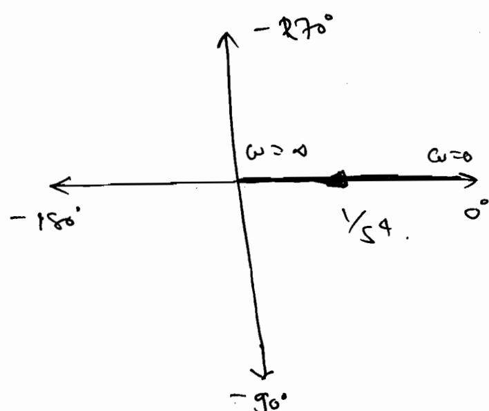
Note: Whenever poles are added to the origin the total plot shifted  $\mp 90^\circ$  in the C.W. direction.
