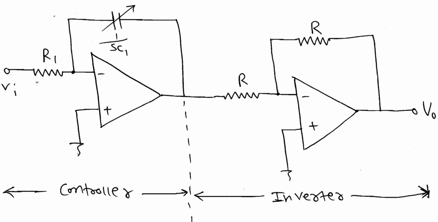
$$\Rightarrow \frac{V_o(s)}{V_i(s)} = \frac{Y_{SC}}{R} = \frac{1}{SCR} = \frac{1}{T_I s} \therefore = \frac{K_I}{s}.$$
