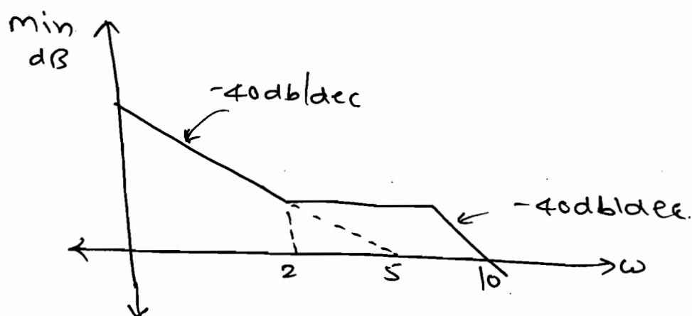
Sol: Initial Slope =  $-40 \text{ dB/dec} = -2 \times 20 \text{ dB/dec}$
