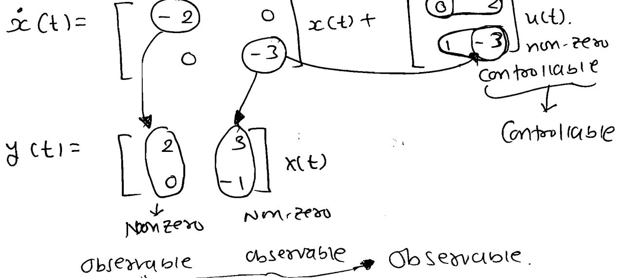
$\Rightarrow$  So, the given system is both observable and controllable.
