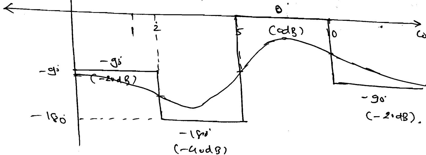
⇒ The Initial Slope of the plot is given by Poles and Zeros located at origin.
