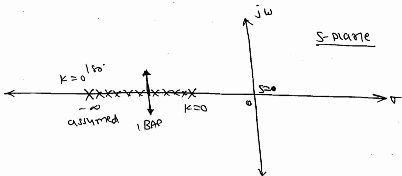
$\Rightarrow$  Whenever there exist a left most side pole to the left most side of that pole there exist a RL branch then there should be a minimum one breakaway point to the left most side of the poles less than zero. When the no. of zeros only.
