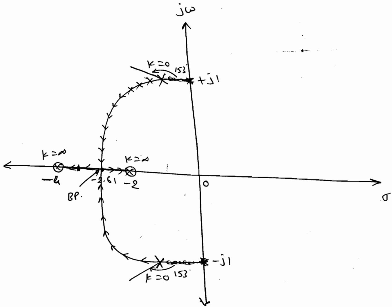
$$\Rightarrow \angle \text{CNI} \Big|_{s=-1+j} = \frac{\angle K \angle 1+j \angle 3+j}{\angle 0 \angle 2j}$$
