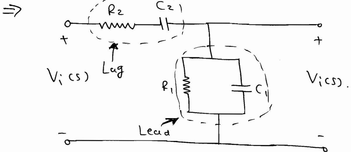
$$\frac{V_o(s)}{V_i(s)} = \left( \frac{1 + \gamma_1 s}{1 + \alpha \gamma_1 s} \right) \left( \frac{1 + \gamma_2 s}{1 + \beta \gamma_2 s} \right)$$
