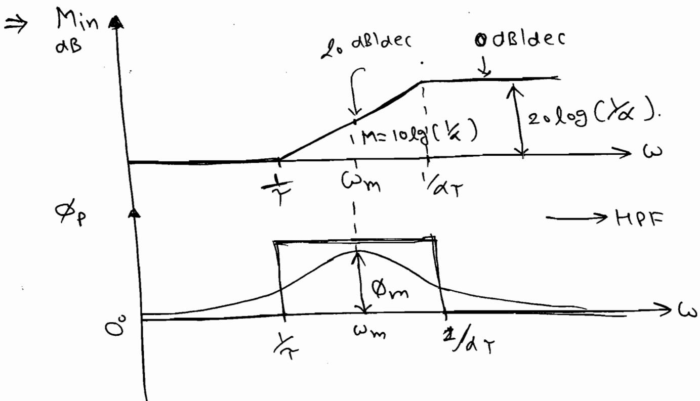
$$\Rightarrow \omega_m = \sqrt{\omega_{c1} \times \omega_{c2}}, \quad \omega_m = \sqrt{\frac{1}{\tau} \times \frac{1}{\alpha T}}$$
