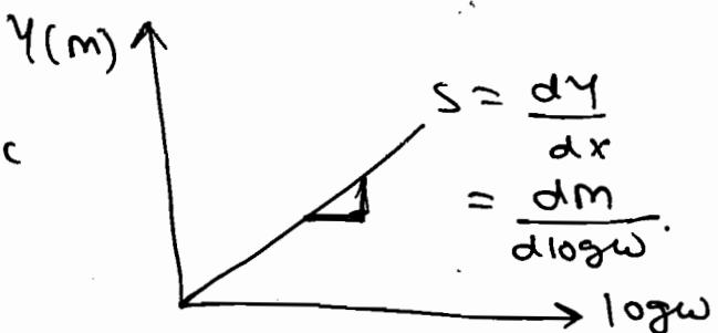
$$M_{\text{in dB}} = 20 \log K \quad \begin{cases} \rightarrow K = 1 \Rightarrow M_{\text{dB}} = 0 \text{ dB} \\ \rightarrow K > 1 (10) \Rightarrow M_{\text{dB}} = 20 \text{ dB} \\ \rightarrow K < 1 (0.1) \Rightarrow M_{\text{dB}} = -20 \text{ dB.} \end{cases}$$
