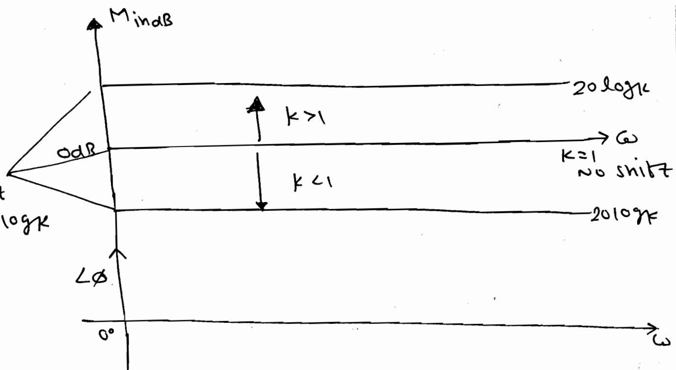
Note: The phase plot is independent of  $K$  value where as the shift in the magnitude plot depends on  $K$  value.
