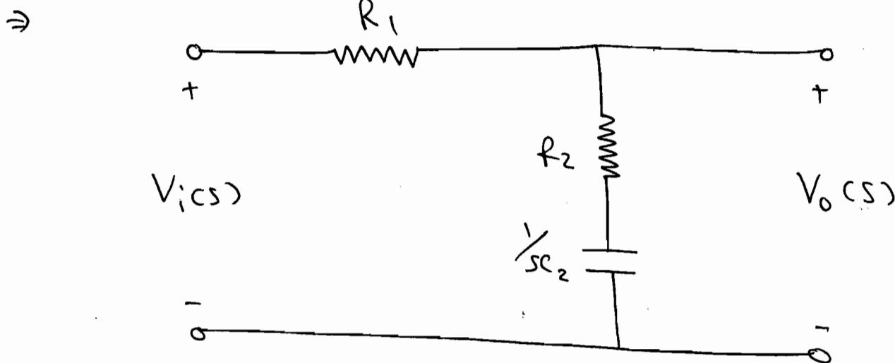
$$\Rightarrow \frac{V_o(s)}{V_i(s)} = \frac{R_2 + \frac{1}{sC_2}}{R_1 + R_2 + \frac{1}{sC_2}}$$
