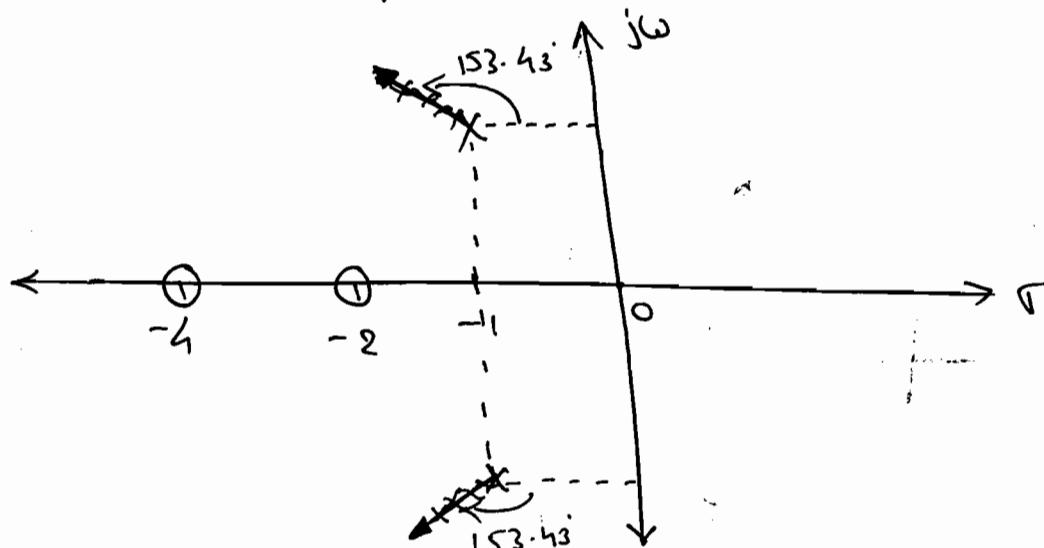
$$\begin{aligned} \angle_{GH} \Big|_{s=-1+j1} &= \frac{\angle K \cdot \angle 1+j1 \cdot \angle 3+j1}{\angle 0 \cdot \angle j2} \\ &= \frac{0^\circ + 45^\circ + 18.43^\circ}{0^\circ + 90^\circ} \end{aligned}$$
