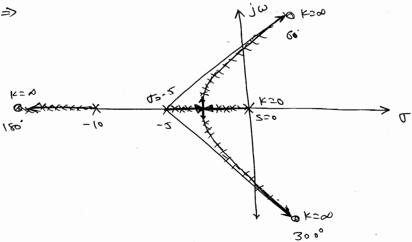
$$\Rightarrow \text{At Collision } +\frac{180}{n} = \pm \frac{180}{2} = \pm 90^\circ.$$
