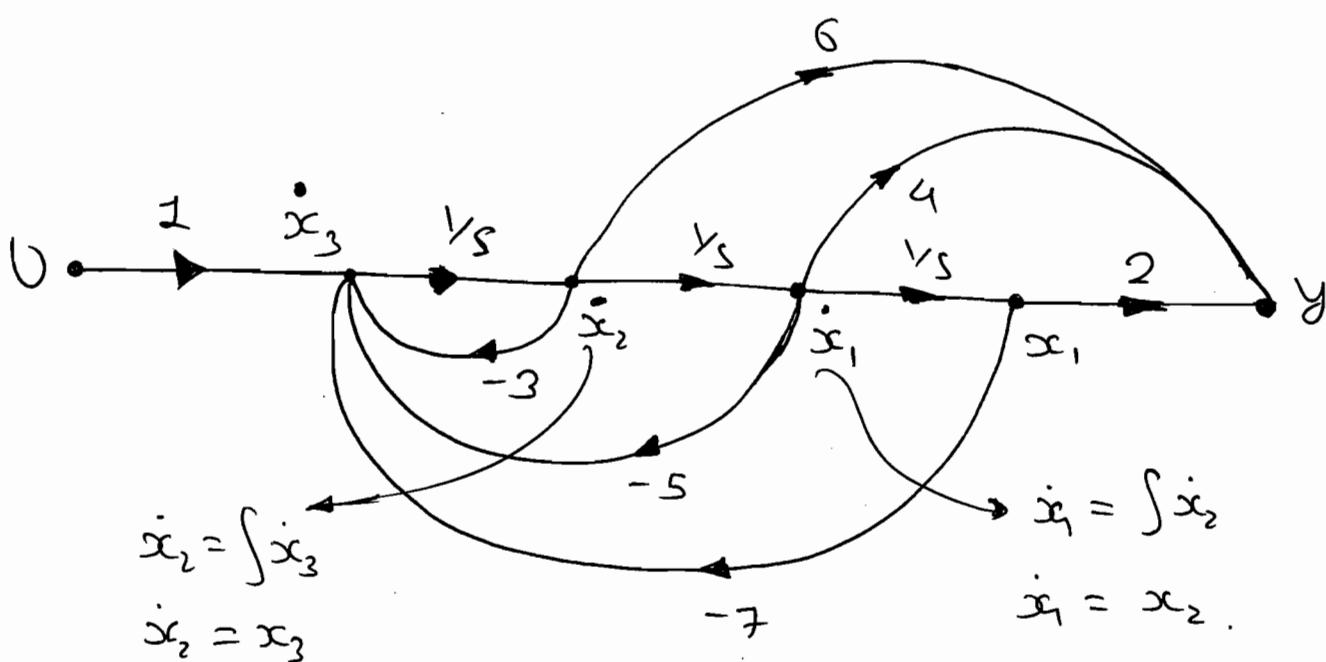
$\Rightarrow$  To select the mode as a state variable, the incoming branch to that particular node must be a integrator, like
