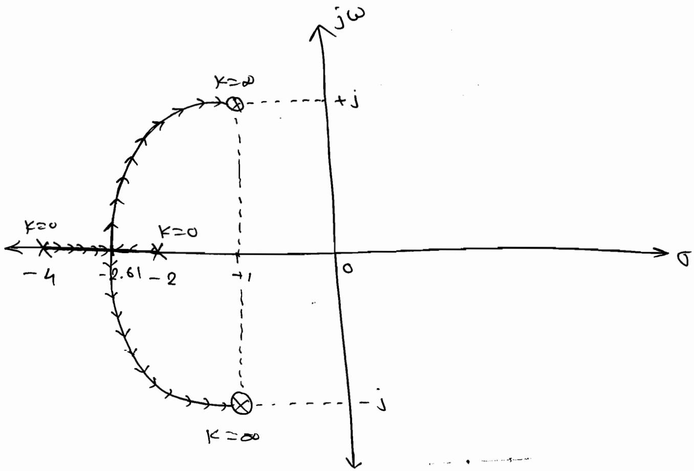
Note: The correct root locus diagram is the one that it should be symmetrical about the real axis and the direction of the root locus branch is from pole to zero when K is increase from 0 to ∞.
