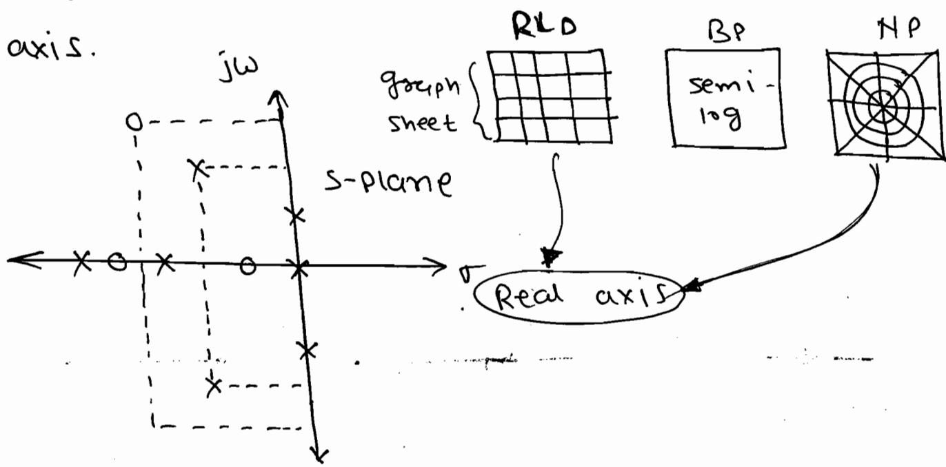
→ The summ. not depends on poles and zeros location, it depends on the graph sheet and on which the plot is constructed the NP (Nyquist Plot) also symm. about the real axis but not Bode plot because the bode plot drawn on non-linear graph sheet (semi-Log).
