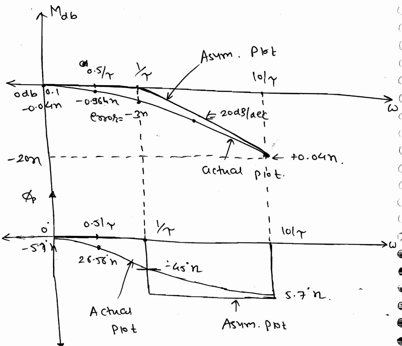
$$\Rightarrow \text{Error} = \underbrace{\text{Actual value}}_{\text{TF}} - \underbrace{\text{Asum. value}}_{\text{Plot}}$$
