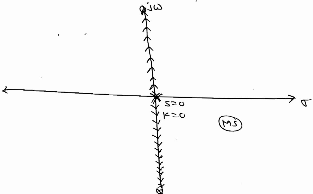
Note: The above system is Marginal Stable for all values of  $k > 0$ . To make it stable we required to add a finite zero in the left side.
