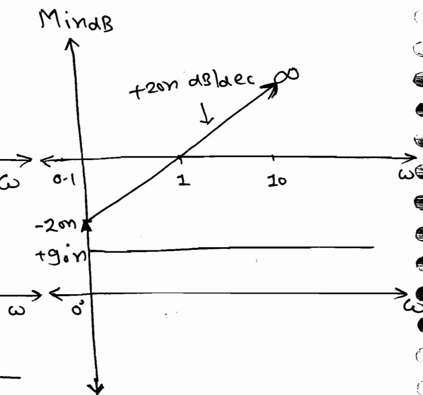
$\Rightarrow$  Whenever the transfer function consists of poles and zeros at origin then the plot starts with a magnitude of  $0 \text{ dB}$  and it should be passes through  $0 \text{ dB}$  line intersect at  $\omega=1$  and extended upto  $\infty$  if no corner freq.
