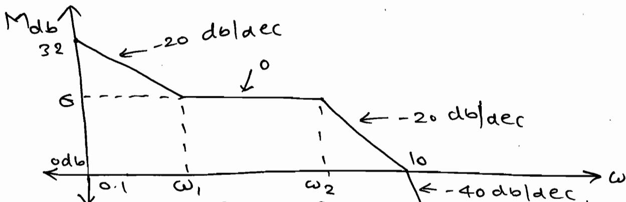
$$\underline{\underline{Slope}} \rightarrow \text{Slope} = \frac{dM}{d\log \omega}.$$
