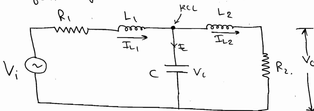
$$\text{Sol: } \text{SV (State Variable)} = \begin{bmatrix} V_C \\ I_{L1} \\ I_{L2} \end{bmatrix}$$
